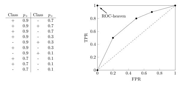
Figure 1.3: Toy example of the results of a probabilistic classifier and the corresponding ROCcurve. The table lists the values for  $p_+$  obtained by the classifier sorted in descending order, together with the true class of each instance. Both classes have cardinality 10. On the right, the ROC-curve is presented. The diagonal line corresponds to a classifier which is randomly assigning classes to instances. The ROC-curve was constructed following Algorithm 1.
