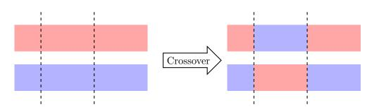
Figure 5.1: Illustration of two-point crossover. On the left, the two parents are randomly divided in three parts by the two cut-off points. The children are constructed by interchanging the middle parts in the parents.
