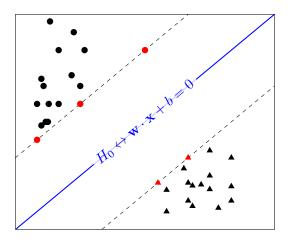
Figure 1.2: Hyperplane  $H_0$  (blue) separating two linearly separable classes of circles and triangles. The support vectors are marked in red.
