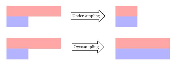
Figure 2.1: Undersampling and oversampling of an imbalanced dataset. In these two examples, a perfect balance between classes is obtained, but not all resampling methods guarantee this result.
