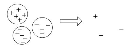
Figure 2.4: Illustration of the execution of CPM. The dataset is clustered, after which only the centers of the clusters are retained in the dataset.
