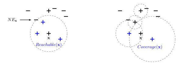
Figure 6.1: Illustration of the  $Reachable(\cdot)$  and  $Coverage(\cdot)$  sets. Each circle contains instances located closer to the center element than its nearest enemy.
