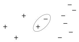
Figure 2.2: Illustration of Tomek links. The elements contained in the ellipse form a Tomek link, as they belong to different classes and are closer to each other than to any other instance.
