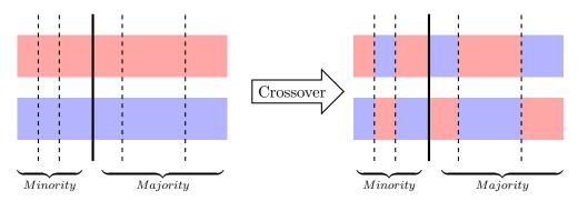
Figure 5.2: Illustration of five-point crossover as used by  $GGA_{Imb}$ . The third cut-off point is always chosen as the division between the minority and majority classes.
